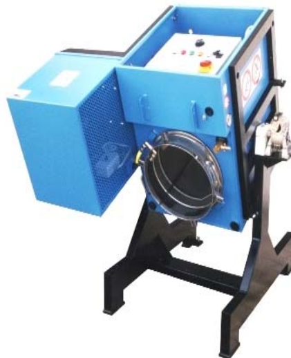
Tilting system and manually clean out distillation vessel
