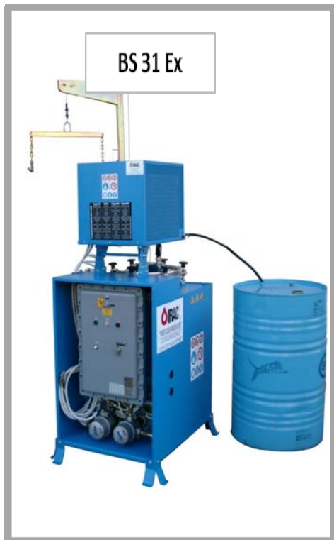
AV system with clean solvent receiving tank
