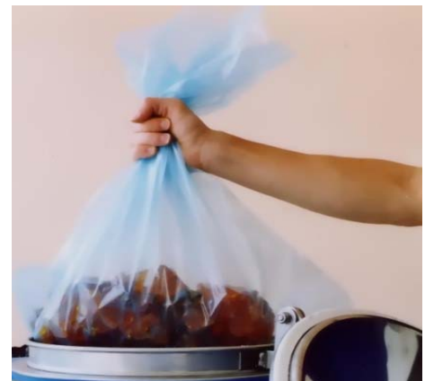
Easy sludge removal using Nylon bag
