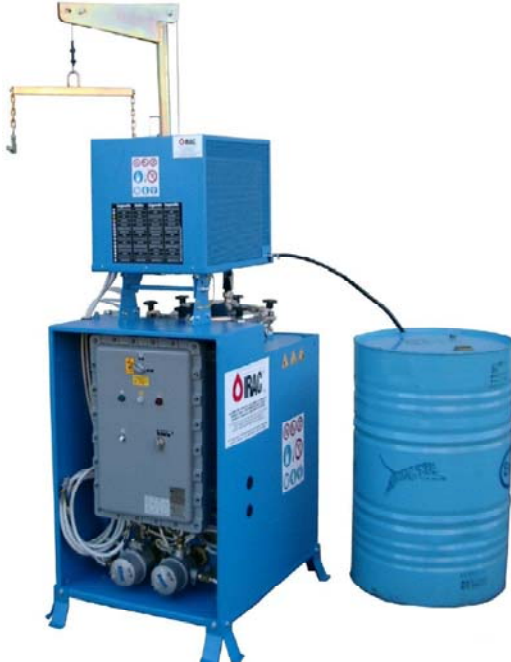
AV system with clean solvent receiving tank
