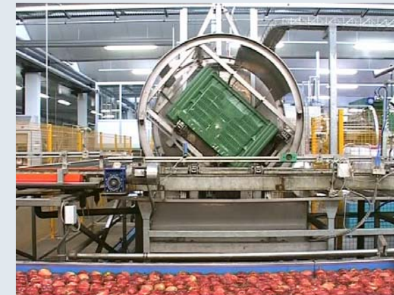
In-feed device ensures empty boxes
